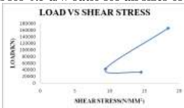
Graph for 0.6 a/w ratio for all sizes of beams Fig 1.18 Graphs for load vs shear stress of a/w ratio of all sizes of beams
