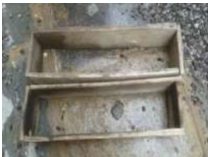
Fig.1.15 wooden mould for medium size beams
